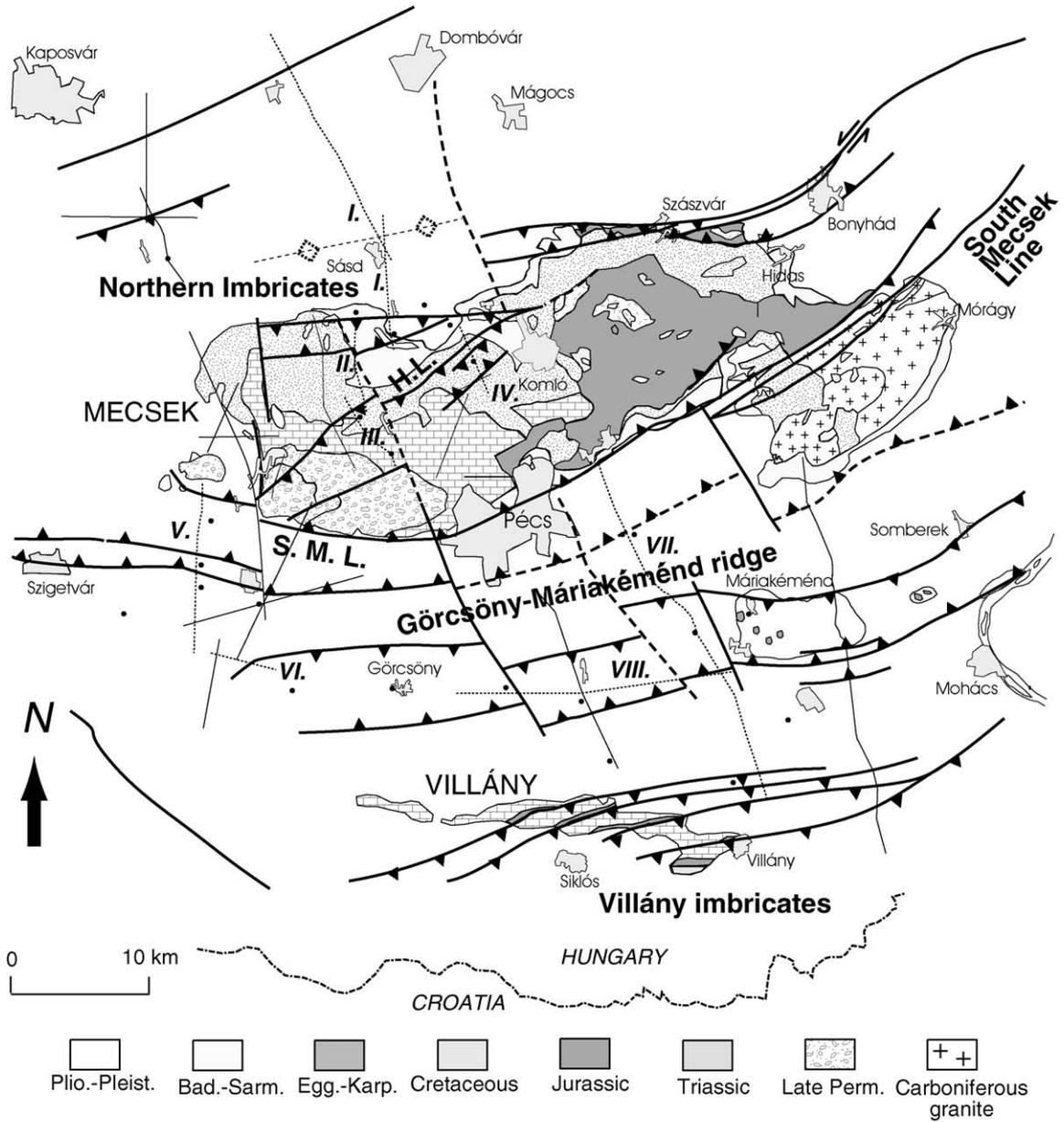
Fig. 2. Structural map of the Mecsek–Villány area based on seismic section reinterpretation (modified after Wórum, 1999). Roman numbers indicate presented sections. S.M.L. = South Mecsek line. H.L. = Hetvehely Line.
