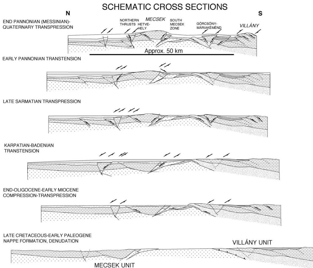
Fig. 16. Structural evolution of the Mecsek–Villány area. Schematic cross sections are roughly balanced sections for the main Tertiary deformation episodes (basic requirements are not met because of large strike-slip motions). Crosses: Mecsek basement. Small dots: Villány basement. Tiles: Mesozoic cover. Coarse dots: Paleogene. Light shading: Early Miocene. Grey shading: Middle Miocene. White: Late Miocene–Pliocene (Pannonian s.l.).
