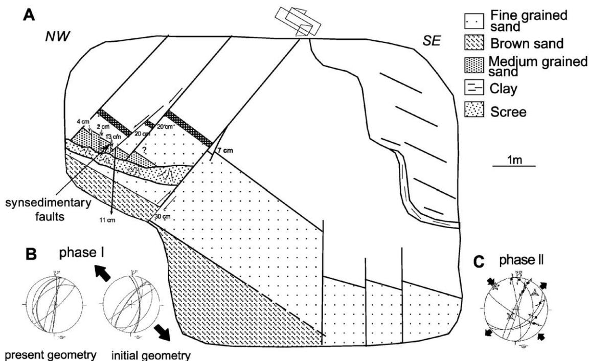
Fig. 9. Máza II (outcrop no. 2). Sketch (A) and stereographic plots (B, C). Data taken from Benkovics (1997). Same legend as in Fig. 7. Elongation directions in B are inferred after backtilting around measured bedding dip value.
