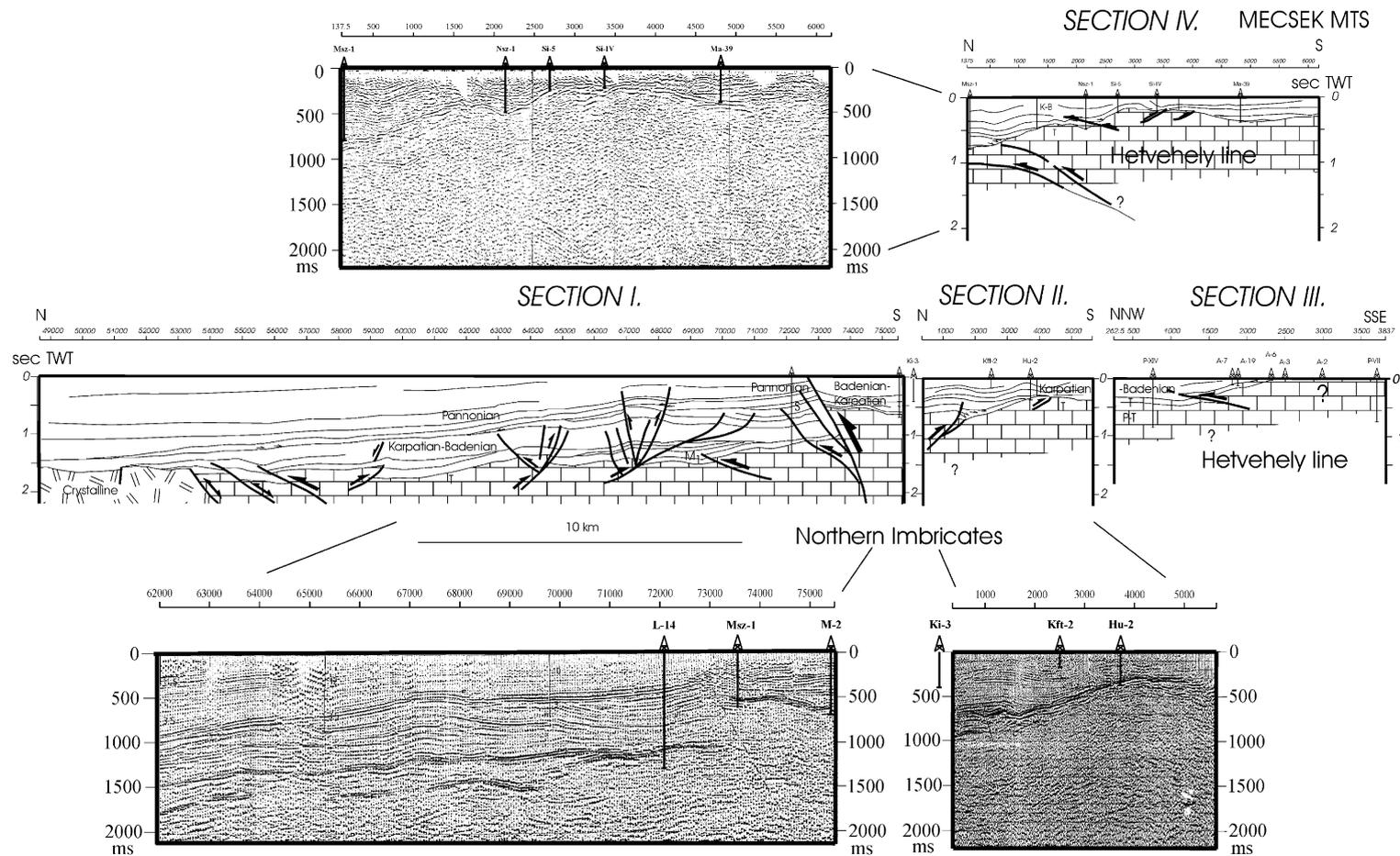
Fig. 4. Seismic section interpretations across the northern part of Mecsek Mountains, after Wórum (1999). Small numbers indicate reference points. Vertical scale in Two Way Travel times. The main body of Mecsek Mountains is towards the south (right) of the sections. S: Sarmatian; K–B: Karpatian–Badenian; M<sub>1</sub>: Early Miocene; T: Triassic; P–T: Permian–Triassic. Boreholes marked as small derricks. Thin lines indicate the portions of lines illustrated by original seismic profiles.
