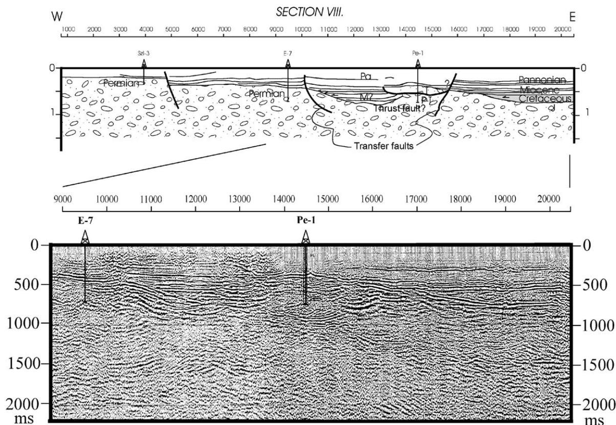
Fig. 6. Seismic section interpretation between Mecsek and Villány Mountains, after Wórum (1999), slightly modified. Small numbers indicate common reference points. Vertical scale in Two Way Travel times. Pa: Pannonian s.l., Late Miocene–Pliocene; M: Miocene; J: Jurassic; T: Triassic; P–T: Permian–Triassic. Boreholes marked as small derricks. Thin lines indicate the portion of line illustrated by original seismic profile.
