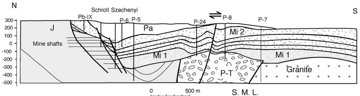
Fig. 15. Geological section at Péccszabolcs (location of section in Fig. 7). Redrawn and slightly modified after Hámor (1966). The section was constructed after exploration wells and coal mine shafts, tunnels. J: Jurassic coal measures; P–T: Permian–Triassic; S.M.L.: South Mecsek line; Mi 1: Early Miocene; Mi 2: Middle Miocene; Pa: Pannonian, Late Miocene. A Pannonian syn-sedimentary extension and a post-Pannonian inversion, thrusting are seen on the section.
