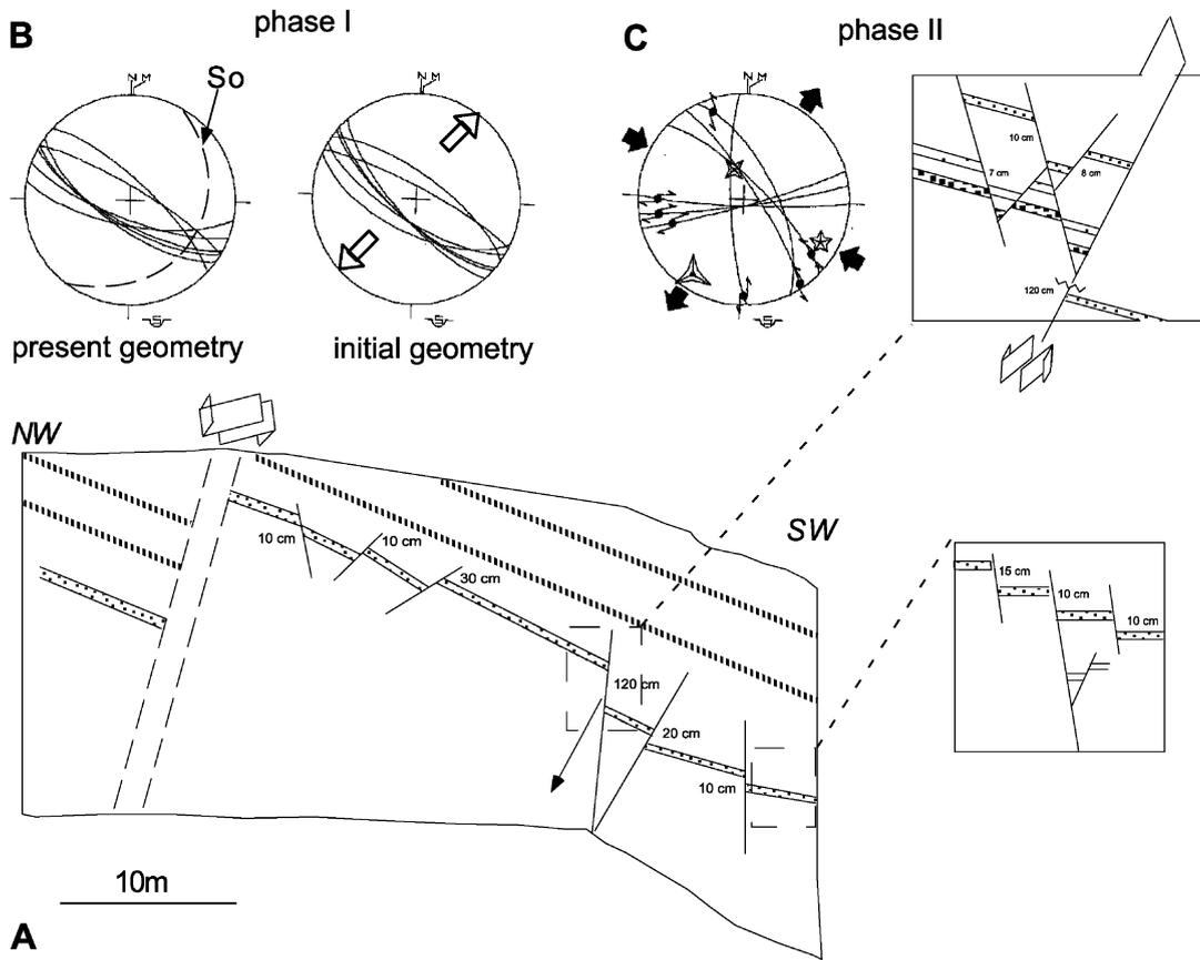
Fig. 10. Rác-hegy (outcrop no. 3). Sketch (A) and stereographic plots (B, C). Some layers are drawn to highlight the syn-sedimentary faulting. Data taken from Benkovics (1997). Same legend as in Fig. 7. Elongation directions in B are inferred after backtilting around measured bedding dip value ( $S_0$ ). Stress field in C may be a later manifestation of B.
