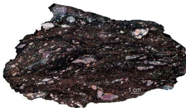
Figure 7. Cut surface of a foliated clay fault gouge deriving from the core zone of the Péter Fault penetrated between 1392.9–1393.9 m in the Eastern Incline
