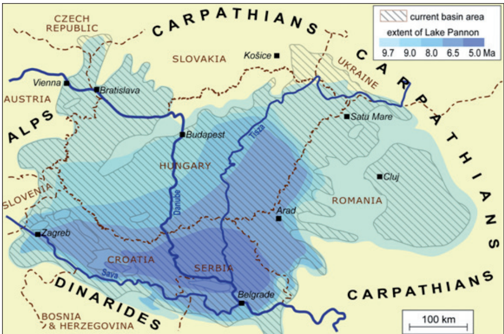
Figure 4.2. Steps of the shrinking of Lake Pannon, together with the main directions of sediment influx (after MAGYAR ET AL. 1999, MAGYAR 2009)
